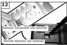
Set dip switches on the Remote Transmitter and Remote Receiver to the same settings. This must be done so the units will communcate properly. If you have other fans you can set to control from one transmitter by setting both receivers the same as the transmitter. If you have more than one fan with remote. You can set the dip switches to different positiosns to have seperate control.
